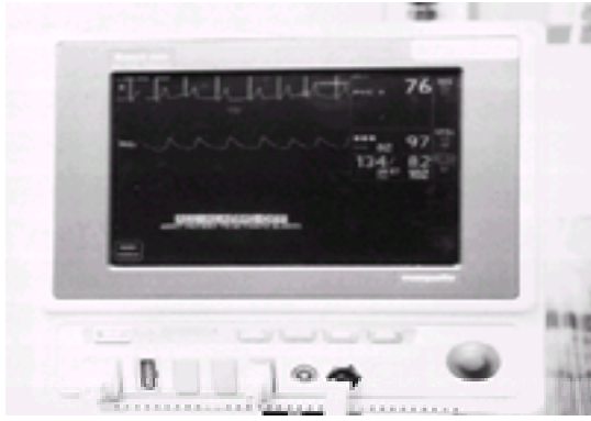
FIGURE 3-4. Continuous display of the electrocardiogram (top waveform) and continuous display of the plethysmographic tracing from the pulse oximeter (second line). Intermittent blood pressure reading is displayed.
